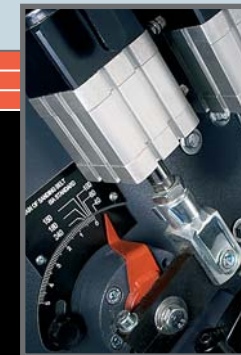
CORRECTION OF WORKPIECE HEIGHT BY GRAIN SIZE OF SANDING BELT
