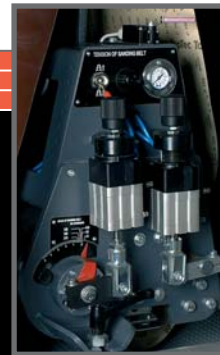
SANDING UNIT C WITH PNEUMATIC ADJUSTABLE WORKING ROLLER
